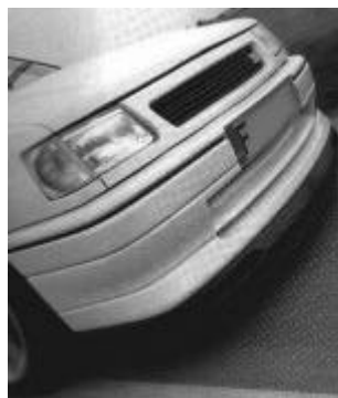
Showing MK2 Nova SRi grille which is the same as the GSi items.
