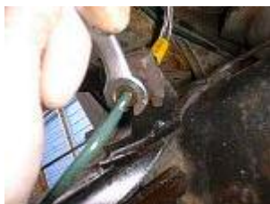
Use a brake spanner to undo brake unions.
