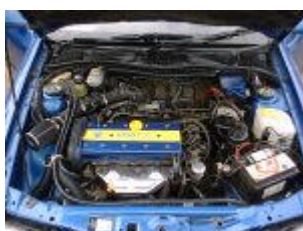
X20XEV DOHC 2L 16v engine.
