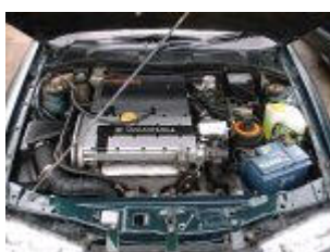
C20LET DOHC 2L 16v Turbo engine.
