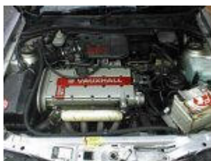
C20XE DOHC 2L 16v engine.
