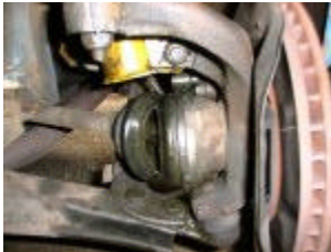
A split CV boot on the front driveshaft.
