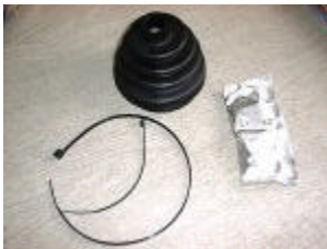
An after market CV boot kit with CV grease and boot ties.
