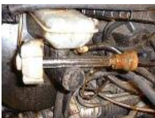
Figure 9 Coolant sensor covered in brown sludge. Sign of either porous head or
