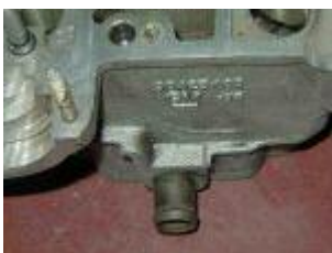
Figure 8 Close up of the oil gallery tube on the side of the cylinder head.
