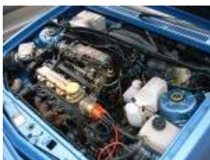
E16SE, a 1.6L 8v fuel injection engine.
