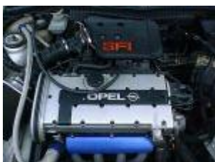
C20XE, a 2L 16v fuel injection engine.
